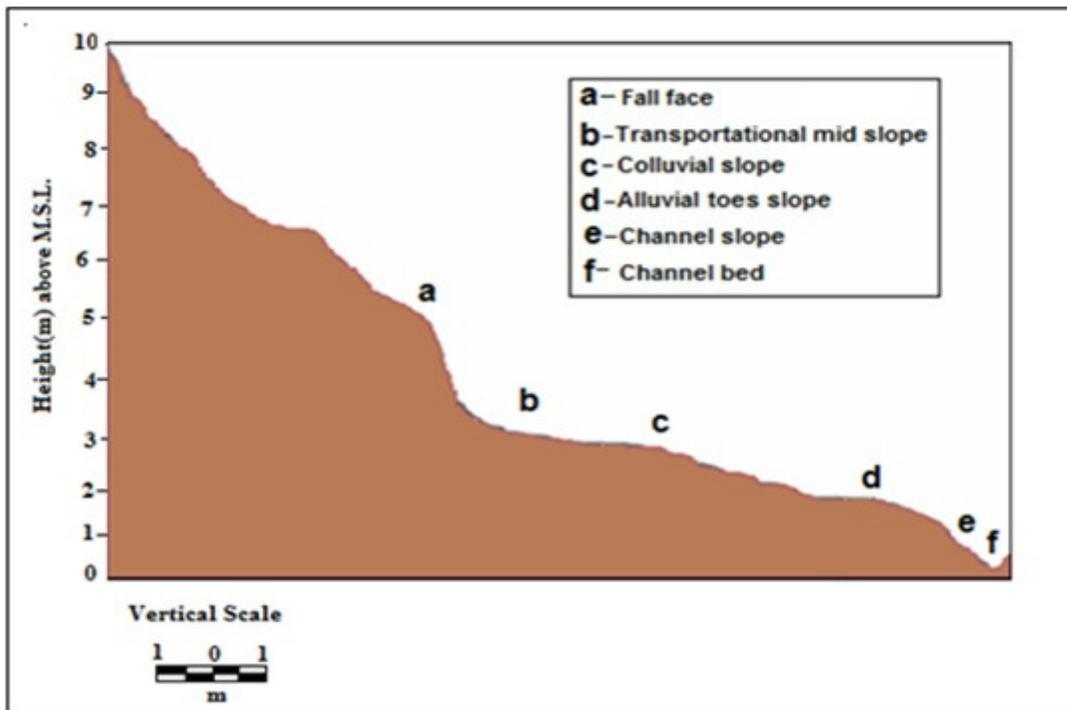
Figure 6: Cross sectional profile to show channel slope variation at Rangamati badland region
