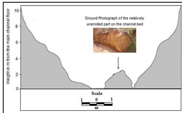
Figure 11: A profile across a gully at Gangani gully area
